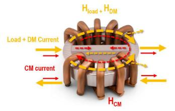
This COMBICHOKE approach can even be combined with VACOCOIL winding optimization to achieve superior performance. The patented VACOCOIL design involves solid copper bars instead of the usual parallel windings of individual copper wires. This VACOCOIL winding design offers significantly improved attenuation at high frequencies (f > 1 MHz) due to lower parasitic winding capacitances.
